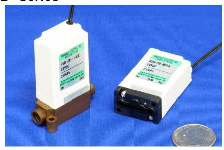
The RVB series is a miniature rocker-style isolation valve suitable for a wide range of manifolds for in vitro diagnostic, analytical and laboratory instruments. The rocker toggles in seesaw fashion, as shown below, and alternately seals the left and right valve seats. Our universal or bi-directional flow path simplifies the manifold designing processes.
